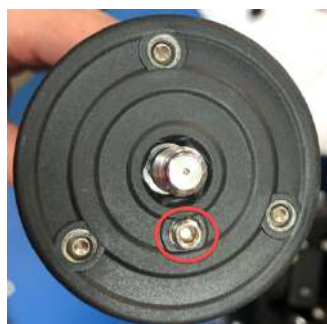
Take out the screw indicated in red to remove the disc from the monopod.
