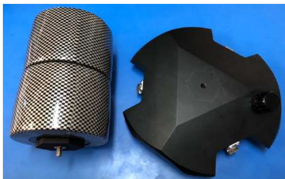
Floats package with mounting screw and 360 lid with mounting point in the middle
