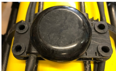
Altimeter accessory installed on the underside of the ROV body
