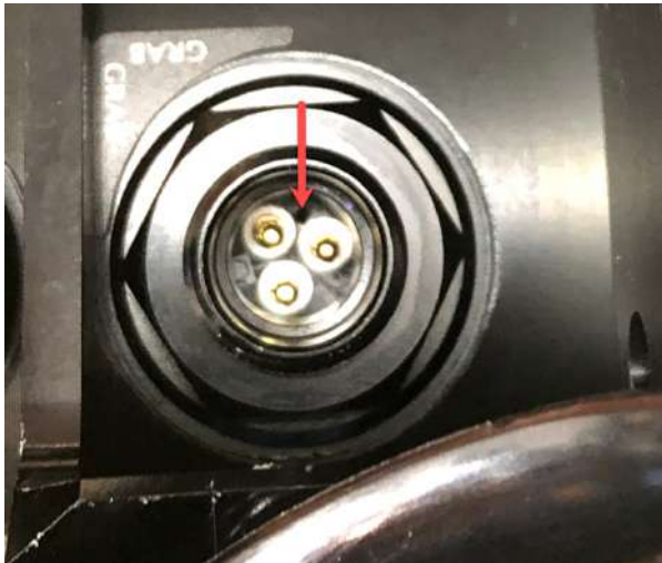
Grabber port. Arrow shows the hole for the grabber plug
