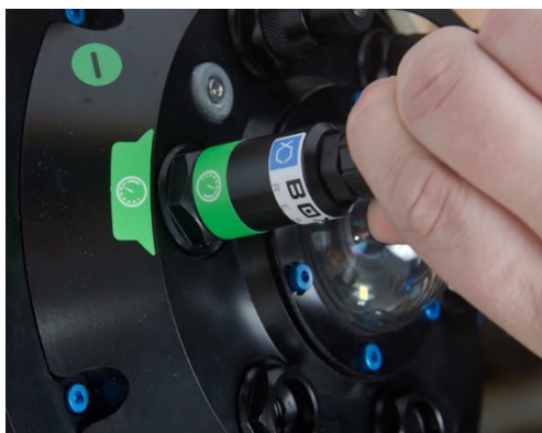
Holding the vacuum hose in place while pressurising the ROV
