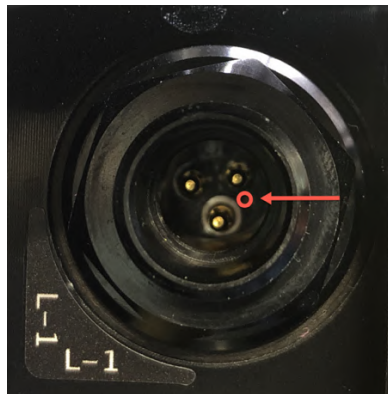
Red circle indicates position of pin hole in light port
