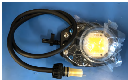
Boxfish LED illumination light assembly
