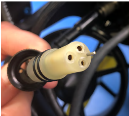
Pin on light penetrator that must line up with hole in light port
