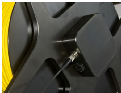
Fibre patch cable connected to tether reel
