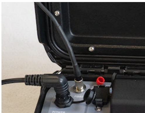
Fibre patch cable connected and secured to Control Station
