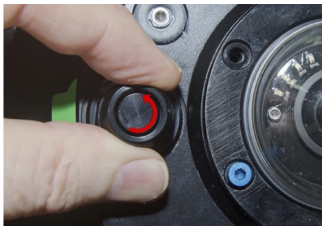
Unscrewing cap from vacuum port
