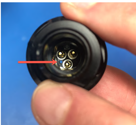
Another view of light port with pin hole visible
