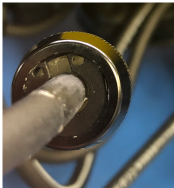
Penetrator nut with clip inside
