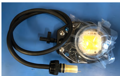
Boxfish LED illumination light assembly
