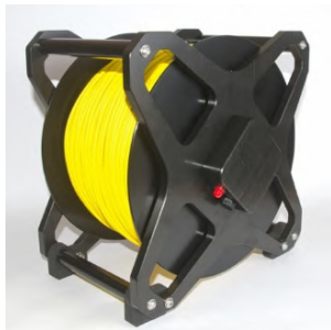
Fibre patch connection point on tether reel covered by red cap
