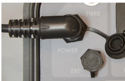
Power cable plugged in and secured with plastic collar
