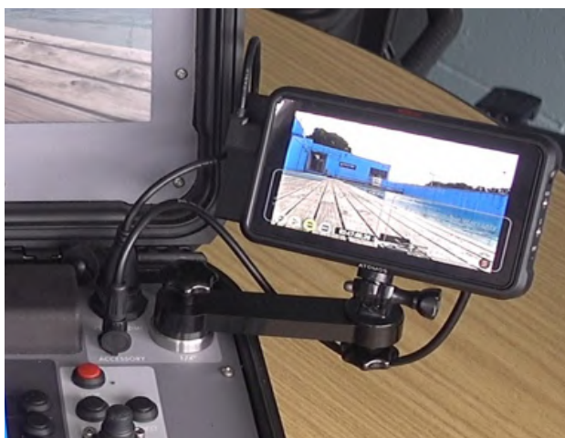
Ninja V installed on Control Station
