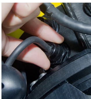
Cap should be finger tight
