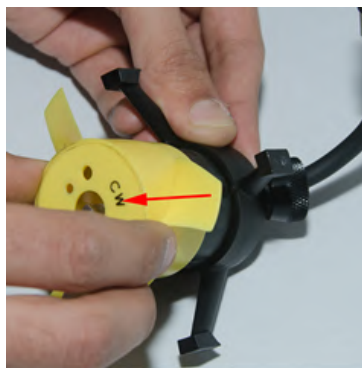
Unscrewing hex head screws Sliding propeller off motor
