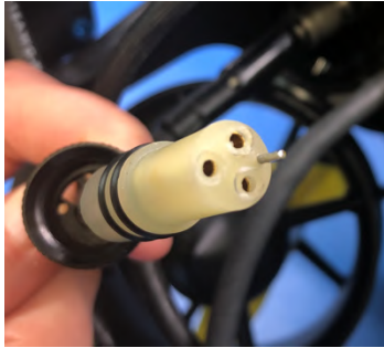
Light penetrator removed from port
