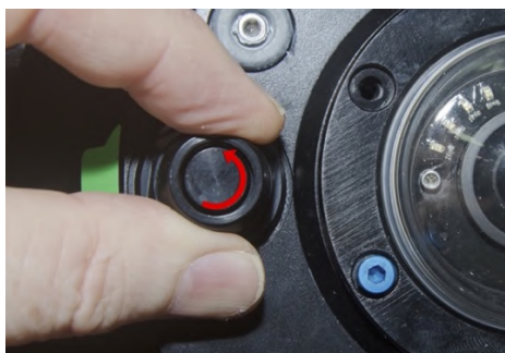
Unscrewing cap from vacuum port
