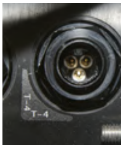
Three pins in the thruster port
