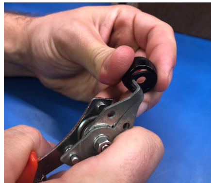
Removing clip with circlip pliers
