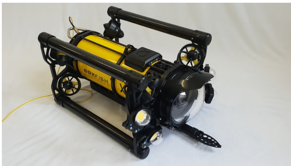
Boxfish ROV with Reach Robotics high-strength grabber
